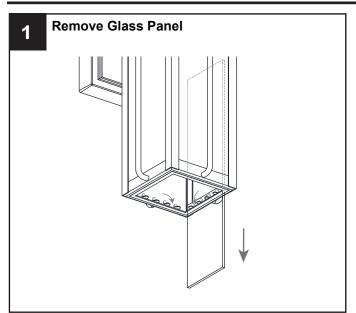
Reverse above steps to reinstall the replacement Glass Panels onto fixture.
