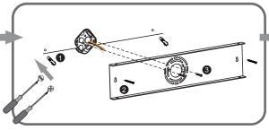
For drywall installations, insert wall anchors into the holes. Otherwise, secure crossbar assembly using self-tapping screws. Then, fully tighten the outlet box screws.
