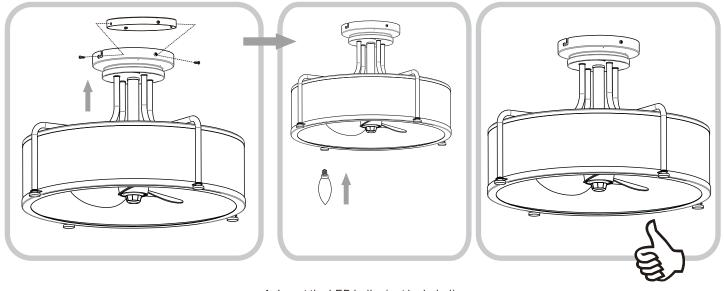
A. Insert the LED bulbs (not included) into the socket and thread in place.
