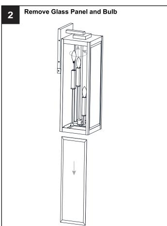
Reverse above steps to reinstall the replacement Glass panels onto fixture.
